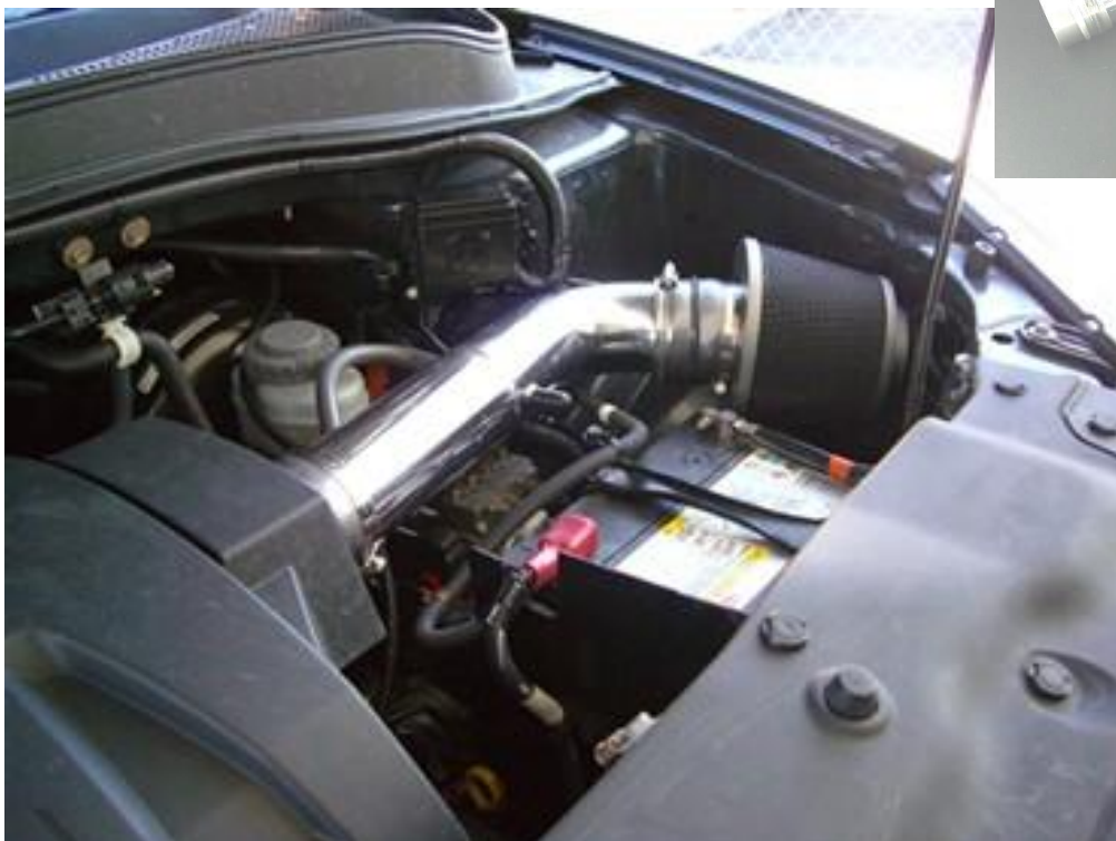
2005 Pilot V6 SW intake install shown
