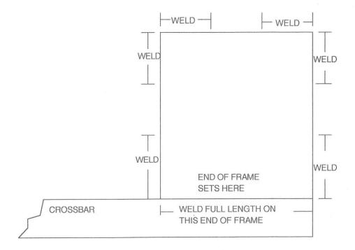
LOOKING DOWN AT THE TOP OF CROSS BAR WITH BOTH BRACKETS, DRIVERS SIDE. DO NOT MAKE CONTINUOUS WELDS
