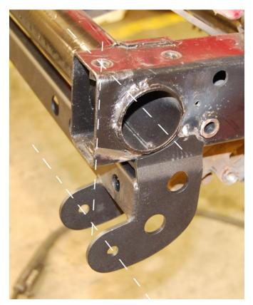
and lightly set the vehicle on the ground to compare it to the diagram below. Do not tighten bolts. Adjust the frame bracket as needed on the frame to make it similar to our diagram.
