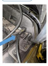
4. Connect hose to other side of Tee making sure to rout under cross support
