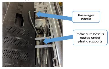
6. Rout hose from passenger nozzle to driver nozzle. Cut hose at tee making sure there is enough slack for press fit to be secured.
