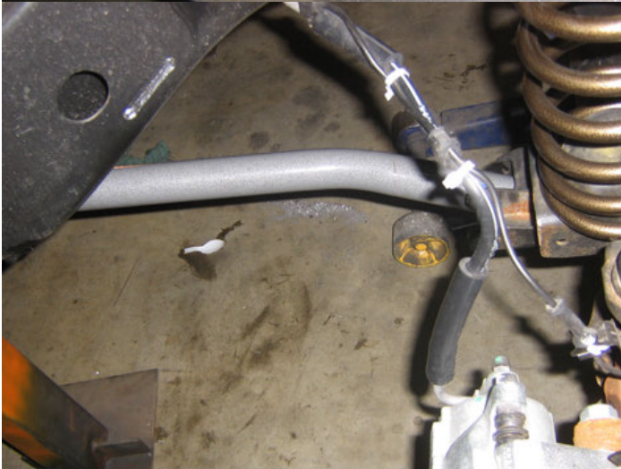
Figure 3 - Shows end of coil rotated into notch
