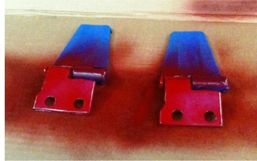
8. After the paint has sufficiently dried, reinstall the modified hinges, cowl and reattach the hood. The hinge holes on the hood side are oversized so you have some adjustability to align the hood with the cowl.
