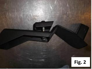
Hold the assembled passenger side bracket against the side of the frame where the factory bumper mount holes are located. The pinch seam of the Jeep tub should set between the bracket and the clamp. (Fig. 3 & Fig. 5) Utilizing a factory bumper side bolt, 'loosely' thread one through the bottom hole of the bracket into the frame. This is to hold the brackets into place while you slide the rear bumper back on. Repeat steps for the driver side.
