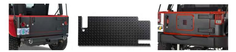
**IMPORTANT:** Warrior only recommends one method of installation. This method includes drilling holes and pop-riveting the tailgate cover into place, and will be the method covered in these instructions. Actual mounting hardware & method are at the discretion of the installer. Any gasket or sealants used are also at the same discretion. All covers are designed to overlay the existing factory tailgate with factory hinges and latches.
