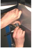
while marking. Once satisfied with the placement of the panel, carefully mark each hole with a permanent marker (making sure not to move the panel). Repeat this process until all panel holes have been marked. The triangular center badge piece is optional and you can leave it off if you prefer. (Fig. 2) INNOVATION SERVICE
