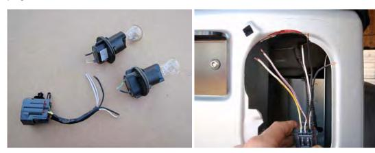
2. Connect your LED light wires to this harness. Below are the wires to join
