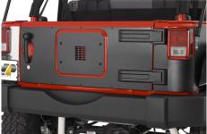
**IMPORTANT:** Warrior only recommends one method of installation. This method includes drilling holes and pop-riveting the tailgate cover into place, and will be the method covered in these instructions. Actual mounting hardware & method are at the discretion of the installer. Any gasket or sealants used are also at the same discretion. All covers are designed to overlay the existing factory tailgate with factory hinges and latches.
