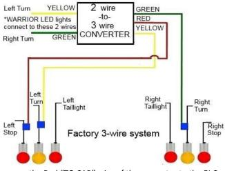
7. You will now connect the wires for the input (3-wire) side of the converter (Refer to the diagram below).
