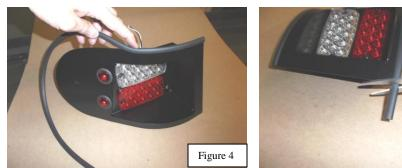
2. Next, remove your factory tail lights. Each light has three mounting studs attaching it to the vehicle. You must access the nuts from the inside of the vehicle cargo area (This is where a "ratcheting" style combination wrench is helpful). There is a small
