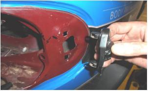
Now, the 3-wire to 2-wire converter must be installed. As mentioned above, it is your responsibility to choose which 4. method you prefer for your wire connections and splices. To install the converter, you should remove the lower plastic threshold below the rear gate by removing the (5) Philips head screws, then gently pulling upward on the plastic trim starting at one end. This is where you can run wires across the vehicle. See Figure 6.
