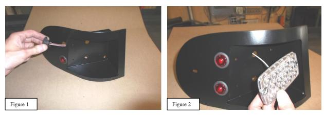
b. Next, mount one Red rectangular S/T/T light, and one White rectangular Reverse light in the undercut portion of the fixture as shown with the provided screws and nuts (you may choose your configuration, with the reverse on the top, or reverse on the bottom, the lights are interchangeable with the mounting locations.) Again, thread the wires through the holes provided from the outside of the fixture as shown in **Figure 2**. The screw holes is the fixture may
