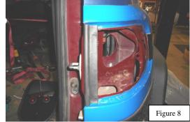
provided for the factory tail light mounting studs. Next, from the inside of the vehicle (in exact order), place a white nylon misalignment space over the threads of the carriage bolt with the angled surface toward the vehicle body. Try to rotate the spacer so that the angle is aligned with the angle of the body. After the spacer is installed, place a washer on the carriage bolt and loosely start the  $\frac{1}{2}$  nut on the threads. Do this for both carriage bolts in this location.
