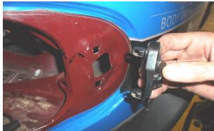
4. Now, the 3-wire to 2-wire converter must be installed. As mentioned above, it is your responsibility to choose which method you prefer for your wire connections and splices. To install the converter, you should remove the lower plastic threshold below the rear gate by removing the (5) Philips head screws, then gently pulling upward on the plastic trim starting at one end. This is where you can run wires across the vehicle. See **Figure 6.**
