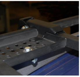
(The padlock tabs should be pointing to the center of the vehicle, as pictured below.)
