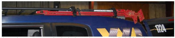
15. The Brackets come equipped with tabs designed to accept a padlock if desired.
