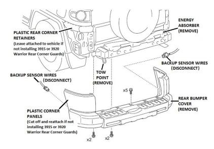
Begin removal of the rear bumper cover taking care not to break any mounting tabs of the plastic corner panels. Remove the rear bumper energy absorber, side stays, side support sub-assemblies, rear bumper bar brackets and the tow point.
