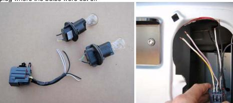
2. Connect your LED light wires to this harness. Below are the wires to join
