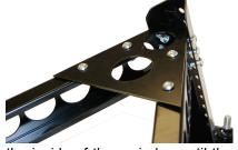
4. Install the tire support shaft (H) onto the assembly. This piece will slide down the inside of the main leg until the top hole in the threaded portion lines up with the top hole in the main leg. Use your 2" long allen bolt to bolt thru the main leg, the tire support shaft, and the vertical tab in the support leg top plate. Use your remaining 1" long allen bolt through the bottom hole in the main leg where the tire support shaft aligns with it.
