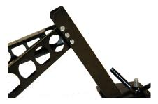
Next, locate the upper leg support plate (A). This will bolt onto the top of the support legs using four of the 1" allen head bolts and lock nuts. Make sure when you install it that the bent tab at the top points up. Again, leave bolts loose until final assembly.
