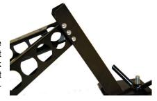
3. Next, locate the upper leg support plate (A). This will bolt onto the top of the support legs using four of the 1" allen head bolts and lock nuts. Make sure when you install it that the bent tab at the top points up. Again, leave bolts loose until final assembly.
