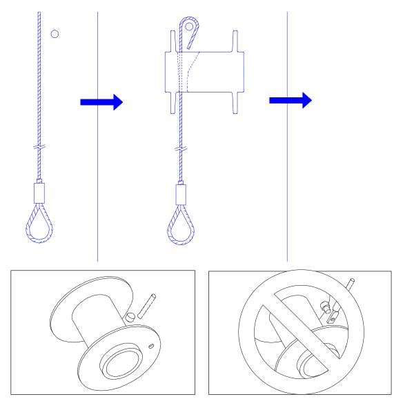
If wire rope has a terminal on the end, it must be cut off before installing.
