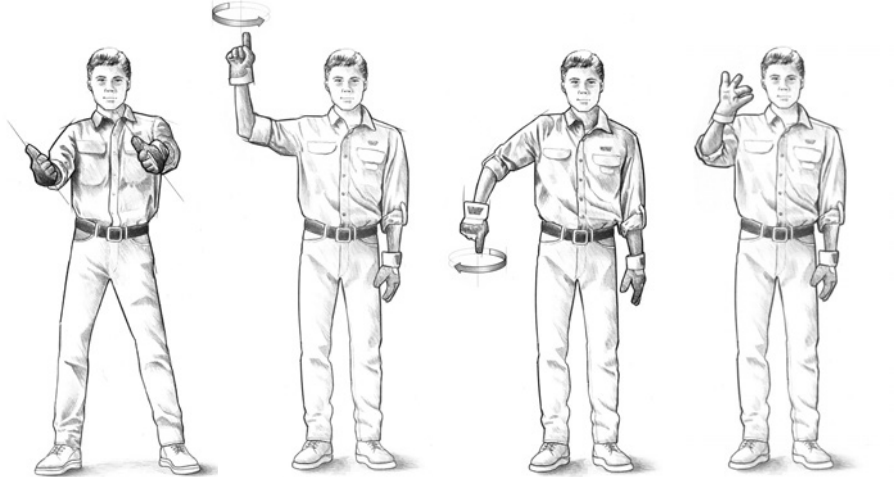
1) Direction of steering Hold your arms out with thumbs up and tilt your hands in the direction you advise the driver to steer.
