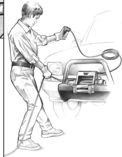
Step 18: REWIND WIRE ROPE. The person handling the wire rope should walk the rope in and not let it slide through the hand and control the winch at all times.
