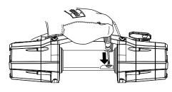
Remove the puck and pull the winch rope through and out of the rope anchor pocket.
