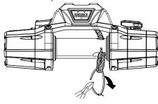
7. Install the 5/16" rope puck in the center of the rope eyelet.
