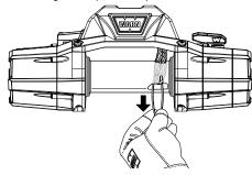
Once the rope has been pulled through, cut and discard the zip tie while being careful not to harm the rope.
