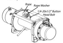
AWARNING Always wind the winch rope on bottom (mount side) of drum.
