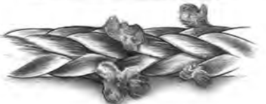
Rope displays two adjacent cut strands— rope should be replaced.
