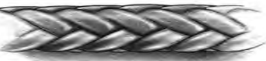
Rope exhibits fiber-set from compression. A slight sheen is visible. This is not a permanent characteristic and can be eliminated by fixing the rope.
