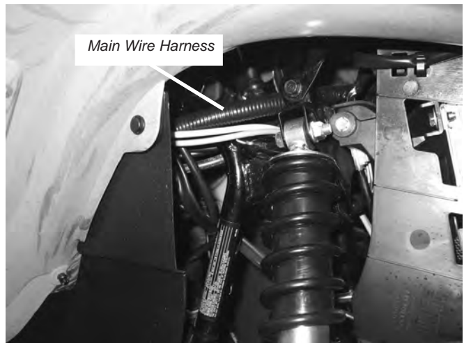
Figure 37 Main Wire Harness - Right Front Wheel Opening
