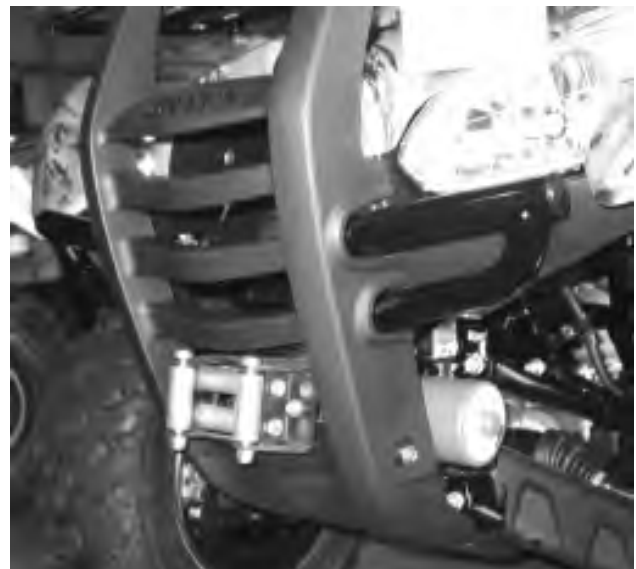
Figure 21 Front Fascia Reinstalled
