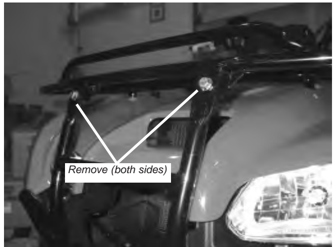
Figure 5 Remove Top Bumper Bolts
