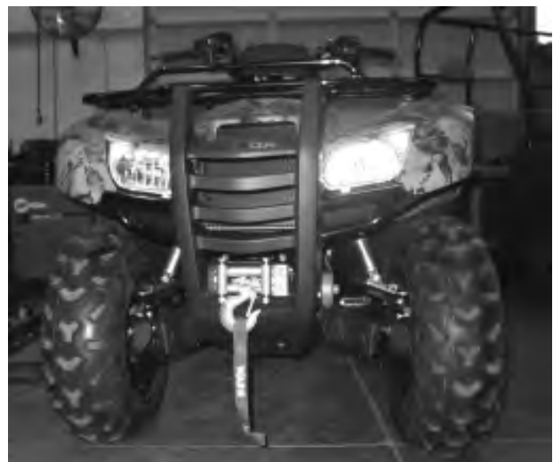
Figure 24 Winch and Mount Installed
