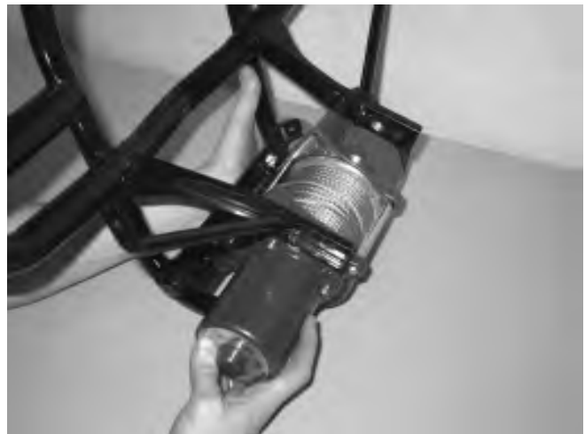
Figure 9 Place Winch in Bumper
