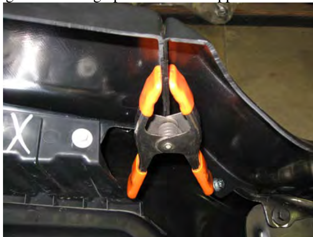
Figure 9: Clamp Top Cap to Center Skirt Piece.
