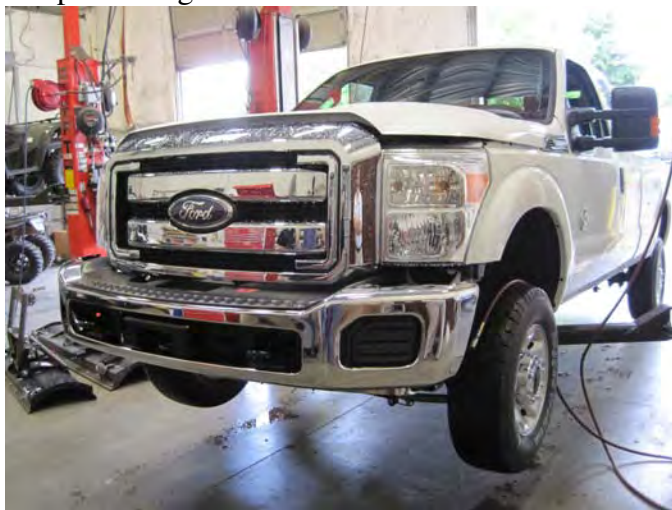
Figure 13: Bumper installed and leveled.
