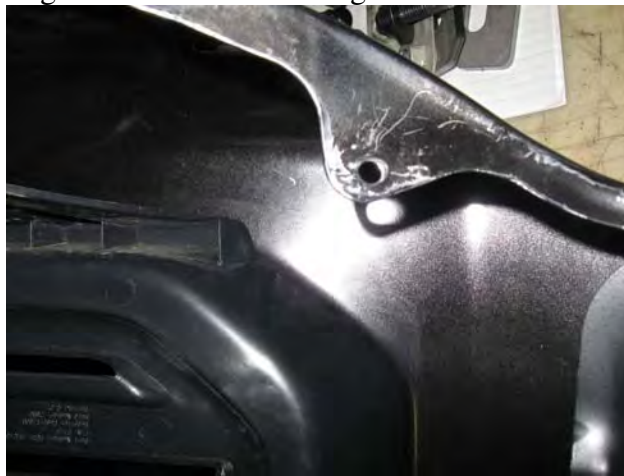
Figure 5: Bumper Flange hole location. (Driver side shown)
