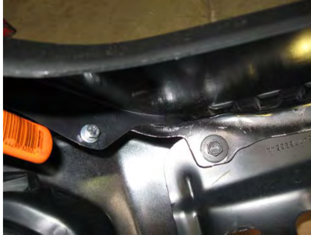
Figure 7: 1/4-20x3/4" Fastener. (Driver side shown)
