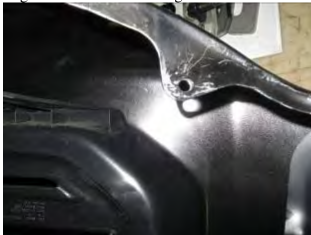
Figure 5: Bumper Flange hole location. (Driver side shown)
