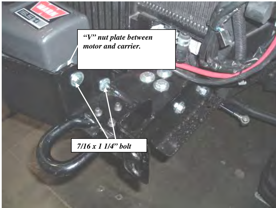
Figure 16: Winch Carrier installed.
