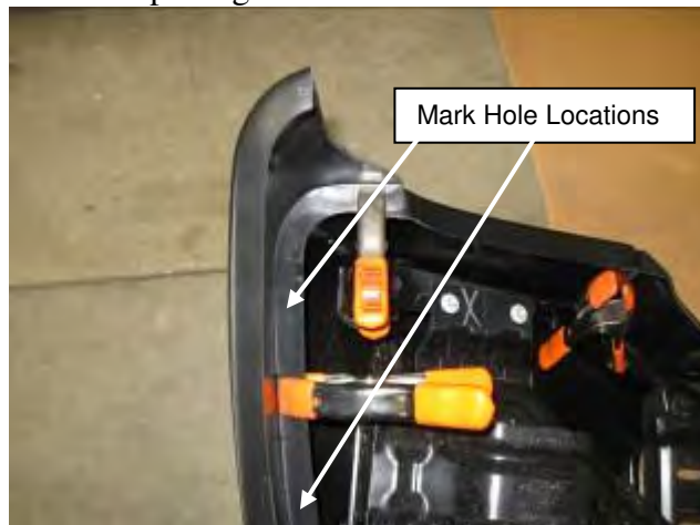
Figure 11: Mark End Cap hole locations from backside.
