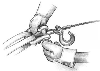
Step 17: DISCONNECT WIRE ROPE. Disconnect from the anchor.
