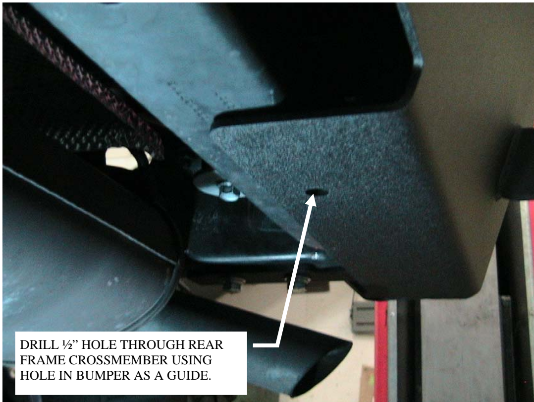
Figure 4: Drill two 1/2" holes into frame crossmember.
