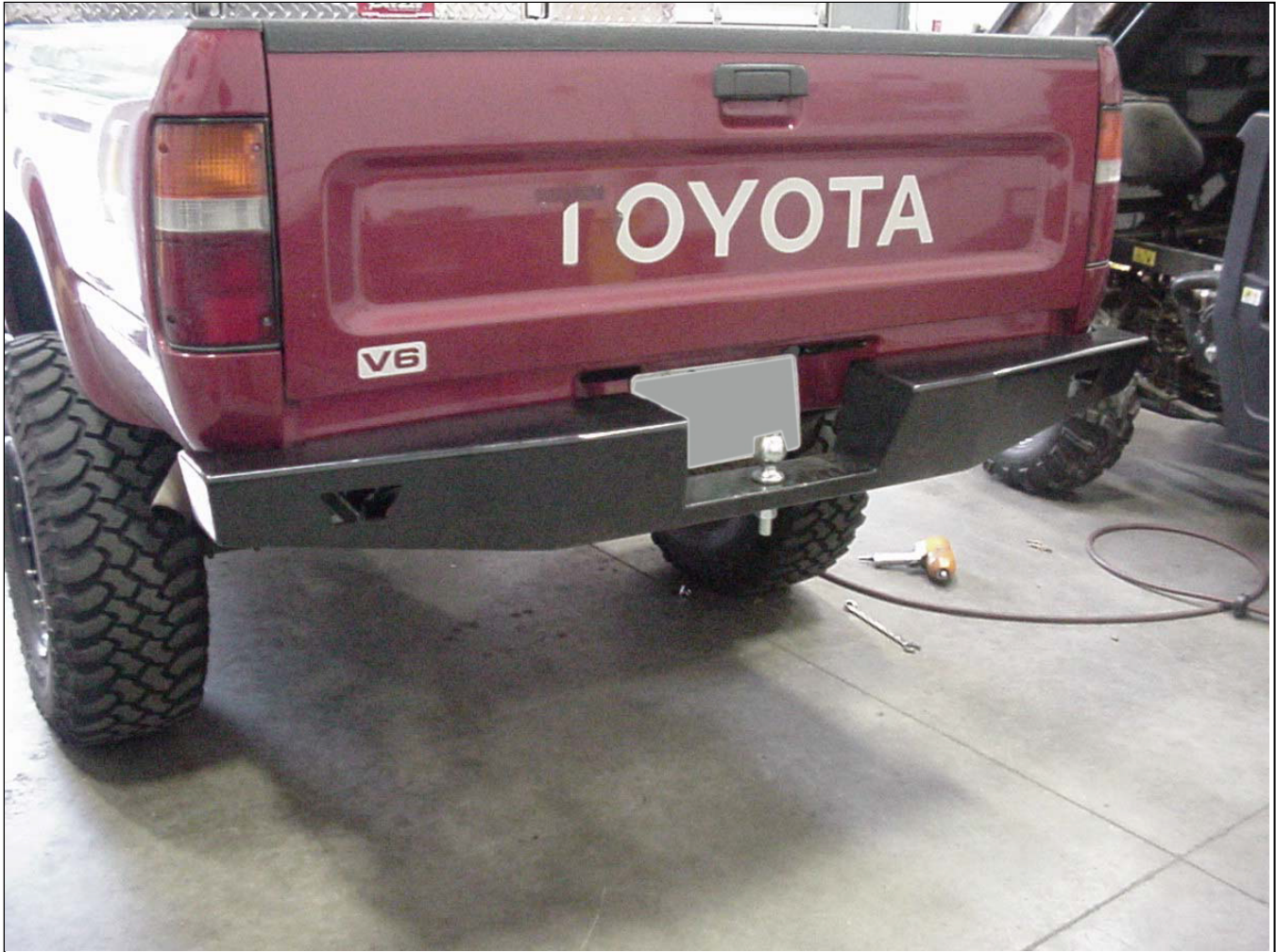
Figure 5, Bumper aligned and mounting hardware torqued.
