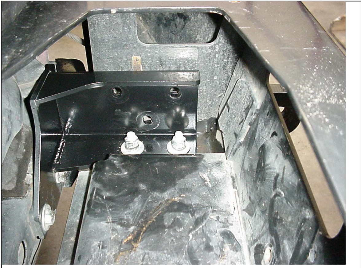
FIGURE 3, BUMPER INSTALLATION USING BOTTOM HOLES IN FRAME BRACKETS.
