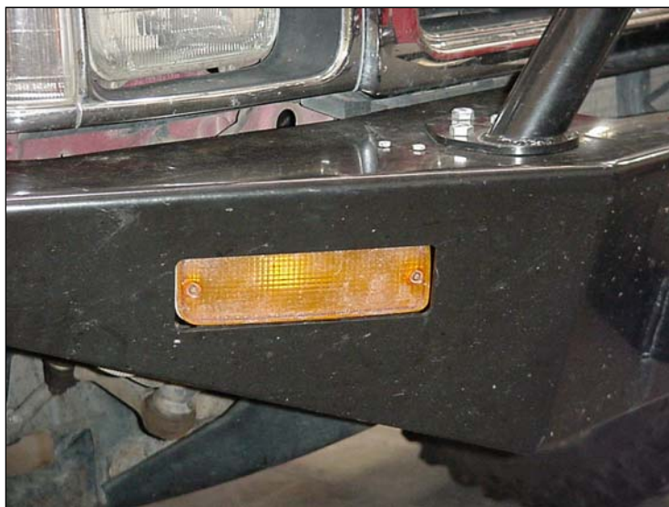
FIGURE 2, TURN SIGNAL INSTALLATION.
