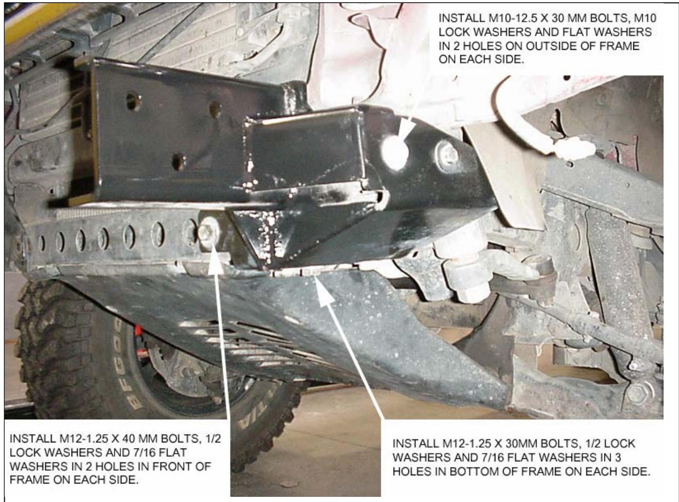
FIGURE 1, FRAME BRACKET INSTALLATION.
