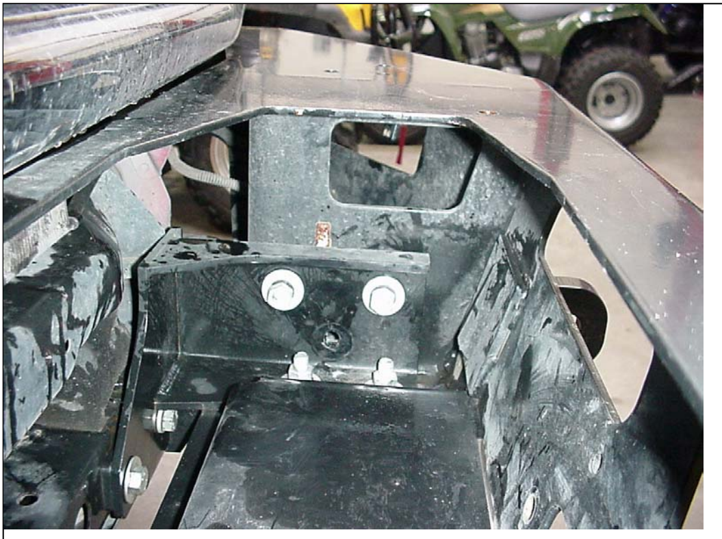
FIGURE 5, BUMPER TO FRAME BRACKET BOLTS.
