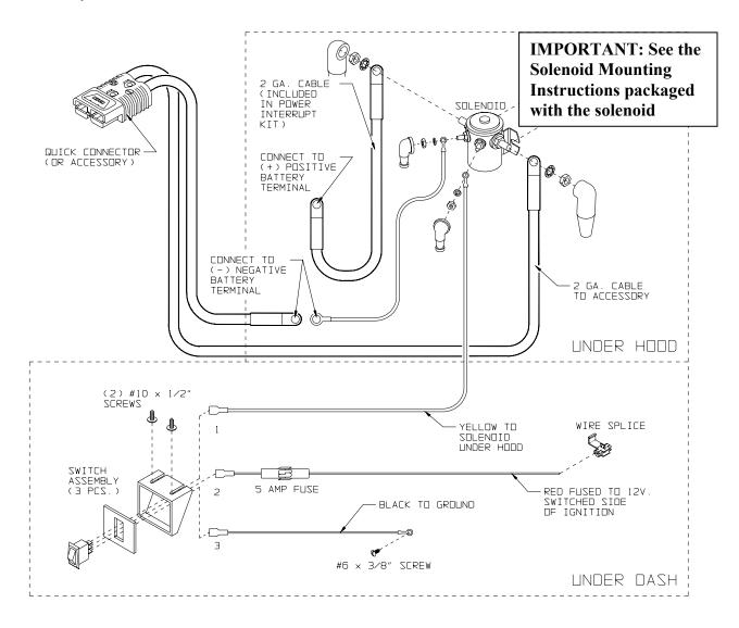
6. Slip a large plastic boot over the red 18" Power Interrupt cable and attach the cable to the remaining large post of the Power Interrupt solenoid. Use the outer nut and washer to secure the cable end. Push the boot over the solenoid post.
