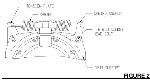
4. Connect the springs to the hooks on the tension plate and the spring anchors. Installation is now complete. WIRE ROPE INSTALLATION NOTE: When installing a new wire rope, unhook the tensioner springs to ease placement of the wire rope end into the rope anchor. After tightening the rope anchor on the drum, re-connect the springs before winding rope onto the drum.
