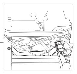
*NOTE: Zip tie cables to vehicle in regular intervals to keep cables secure and in place.*
