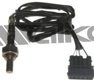
250-24823 VW (6) 1993-94 Heated Sensor
