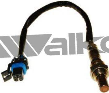
250-24340 BUICK (6) 1996-04 / CHEV (4,6,8) 1996-04 GMC (4) 1996-03 / ISUZU (4) 1997-00 OLDS (6,8) 1996-04 / PONT (6,8) 1996-04 Heated Sensor
