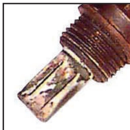
Ethylene Glycol (Antifreeze) Contamination
