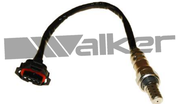
250-24845 PONT (6) 2008-09 Heated Sensor
