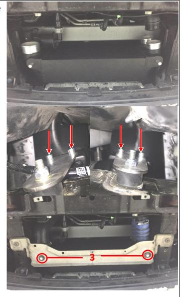
Install the supplied silicon hose and all other charge air hoses to the WagnerTuning intercooler. At least install back the lower cross member. Please note! Don't forget to replace the stock rubber bearing (3)!
