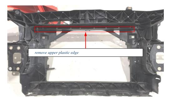
The best would be to insert the WAGNERTUNING intercooler into the radiator support and then mark the exact width and hight of the area which should be removed. Then remove the intercooler and mark yourself a depth of about 40-45mm. Now cut the upper edge with a car body saw or something similar.
