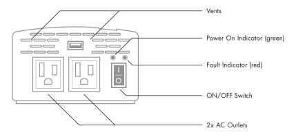
ON/OFF Switch – Controls operation of the inverter. The below indicators operate when the switch is ON.
