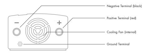
High Speed Fan – The fan turns on when there is a high load or an elevated temperature to keep the inverter cool. Do not block. Keep 2-inch clearance.
