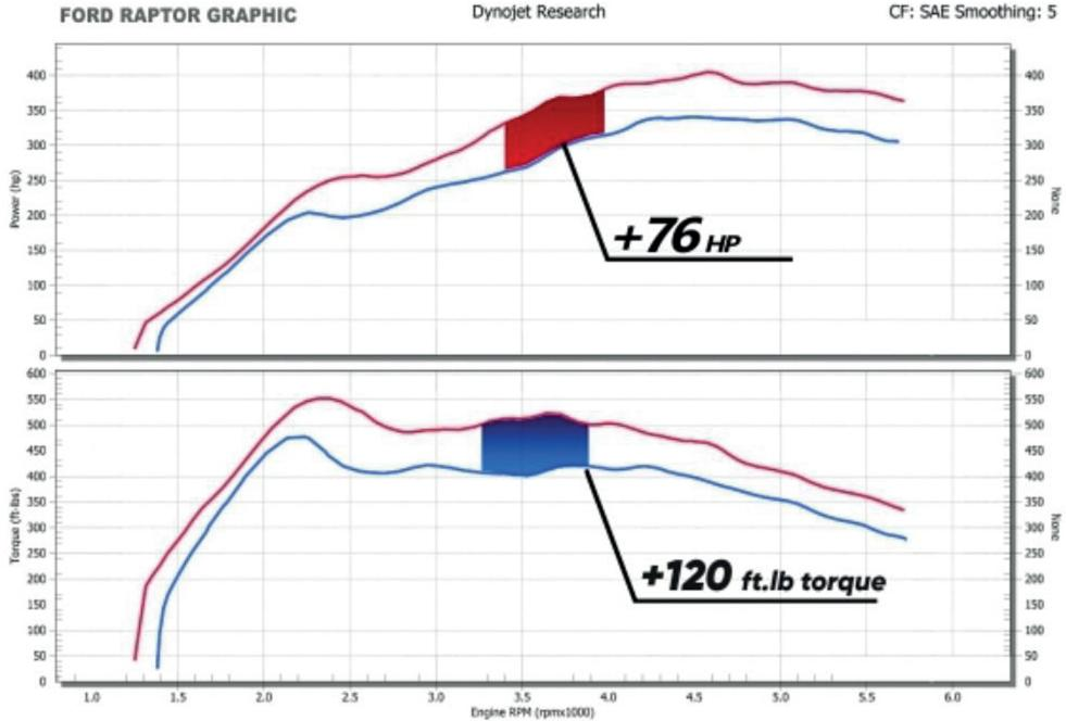
\*Measured on a DynoJet dynamometer.
