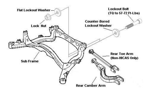
\*Non-HICAS model Shown. HICAS only requires a lockout kit for rear camber adjustment.
