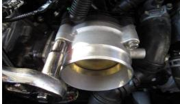
7. Install the 6mm bolts, washers provided. Than install the air duct, MAF sensor harness and negative battery cable.
