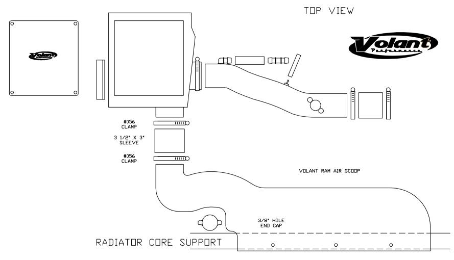
NOTE: REMOVE ALL SIX FACTORY PUSH PINS FROM THE RADIATOR CORE SUPPORT AND REMOVE PLASTIC COVER. PLACE THE VOLANT RAM AIR SCOOP OVER THE CORE SUPPORT AND FASTEN WITH 3 FACTORY PUSH PINS.
