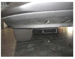
6. Attach the 3.75 x 3.5 sleeve and lower scoop using the #60 clamps
