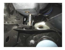
3. Align the rubber bumper with the existing hole on the frame
