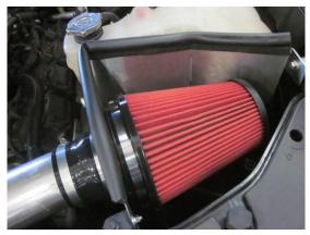
13. Place filter on adapter and tighten clamp using 8mm socket and ratchet.
