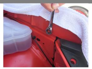
5. Remove bolt from inner fender using 10mm wrench.
