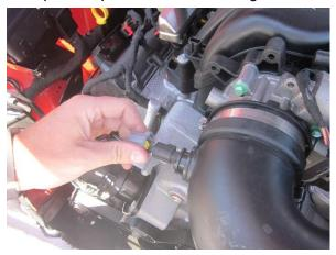
4. Disconnect wiring harness from air temperature sensor (ATS).
