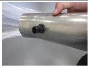
Install supplied rubber grommet into Volant air duct. Install factory ATS from removal step 8 into grommet.
