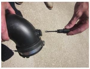
8. Remove ATS from factory air duct.
