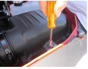
6. Remove bolt securing factory air box to vehicle using 8mm socket and ratchet.
