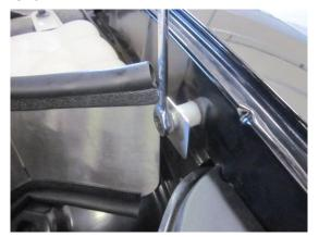
7. Place spacer between shield and inner fender and insert 6mm x 30 bolt with ¼" lock washer and ½" flat washer. Tighten bolt with 10mm socket and ratchet.
