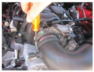
3. Loosen clamp securing factory air duct to throttle body using 5/16" socket and ratchet.
