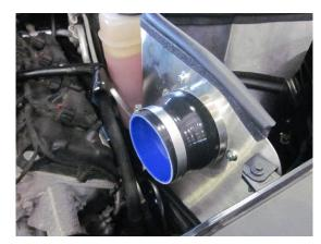
Install reducer onto filter adapter along with #64 clamp placed loosely on large end and #60 clamp placed loosely on small end.
