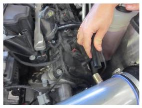
14. Install supplied breather hose onto Volant duct and factory location on engine.
