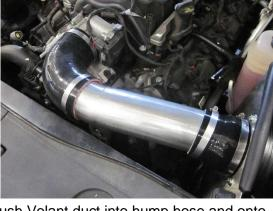
12. Push Volant duct into hump hose and onto throttle body. Adjust duct as necessary and tighten all four clamps using an 8mm socket and ratchet.
