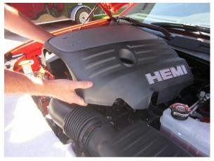
2. Twist off oil cap. Remove engine cover. Reinstall oil cap to keep debris from entering.
