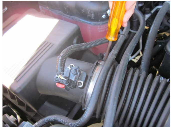
4. Loosen the clamp securing the factory air duct to the factory air box with an 8mm socket and ratchet or nutdriver.
