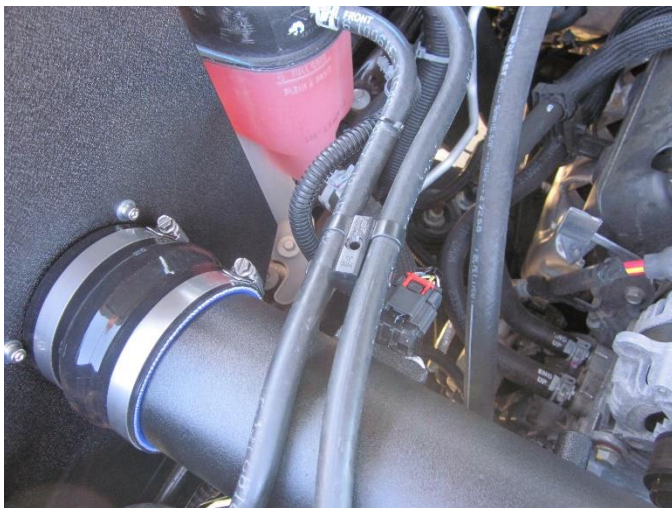
15. Install supplied hose support bracket onto the factory 5/8" lines
