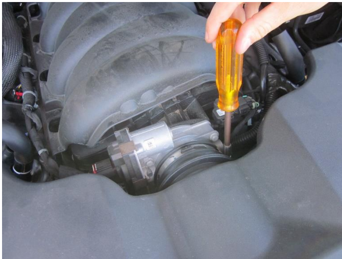
3. Loosen the clamp securing the factory air duct to the throttle body with an 8mm socket and ratchet or nutdriver.
