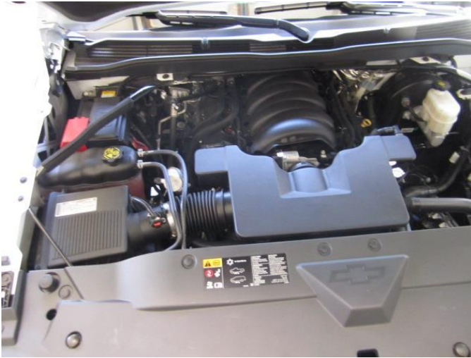
1. Stock air intake system before uninstallation.
