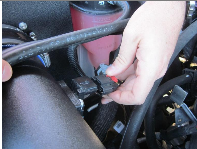
14. Clip MAF sensor wiring harness onto MAF sensor until it clicks. Push red tab down to lock harness in place.
