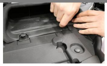
5. Re-install the factory scoop with clips saved from Removal Step 8.
