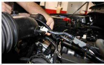
**3.** Disconnect both vent connections from the rear of the factory duct.
