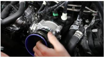
**8.** Install two #56 clamps onto the straight sleeve and place the straight sleeve on the throttle body.
