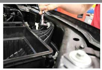
7. Use a ratchet and 13mm socket or wrench to remove the bolt holding the air box to the vehicle. Save bolt for Install Step 4.
