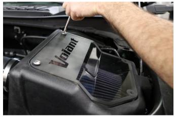
**12.** Install the Volant lid using the provided 4 truss head screws with rubber washers and Philips head screwdriver.
