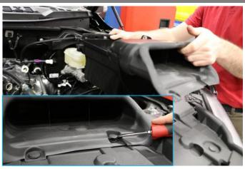
**8.** Remove the two clips holding the factory scoop using a pry tool. Save clips for **Install Step 5**. Remove scoop and air box assembly from vehicle.
