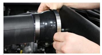
Install one #56 clamp on small end of the reducer, and one #64 clamp on larger end of reducer. Place small end of reducer onto straight end of Volant air duct.
