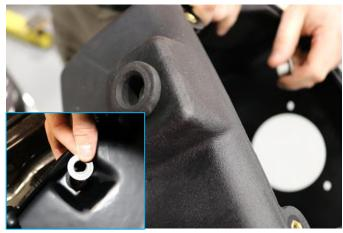
1. Put the metal bushing and rubber grommet from Removal Step 9 into the Volant air box.
