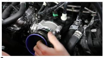
**8.** Install two #56 clamps onto the straight sleeve and place the straight sleeve on the throttle body.
