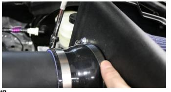
10. Insert the air duct onto the straight sleeve on the throttle body and large end of reducer onto the filter adapter. Adjust Volant air duct to proper fit and tighten all clamps using an 8mm socket or flat head screwdriver. NOTE: Also tighten the filter's clamp at this time.
