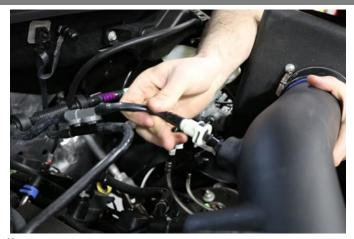
Connect both factory quick disconnects to the Volant air duct.
