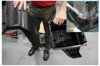
**10.** Remove the bolt holding the factory air scoop to the air box using an 8mm socket. Separate the scoop from box and save it for **Install Step 2**.
