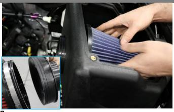
**6.** Install filter adapter onto Volant air filter, then place air filter into Volant air box.
