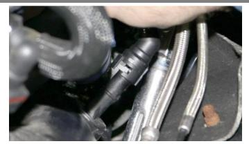
**1.** Unclip the quick disconnect vent hose.
