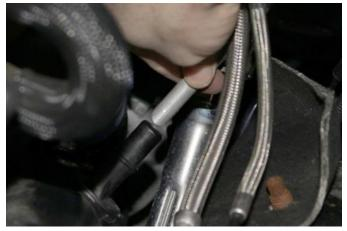
2. Insert vent line fitting with the short side towards the turbo inlet.
