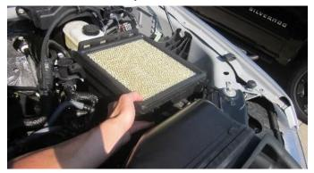
Remove the bottom box assembly by pulling it up and out. Remove the rubber grommet and metal bushing from factory air box. Save for Install Step 4.
