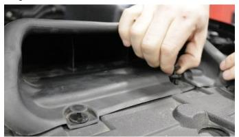
8. Reinstall factory scoop and attach with clips from **Removal Step 6**.
