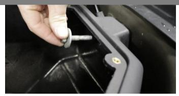
7. Attach the Volant air box to the fender with the bolt from **Removal Step 4** using a ratchet and 13mm socket.
