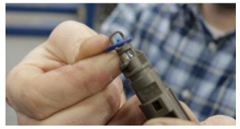
**10.** Remove O-ring from the temp sensor.
