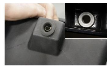
4. Insert the factory grommet from Removal Step7, then install the metal bushing into grommet from inside box as shown.
