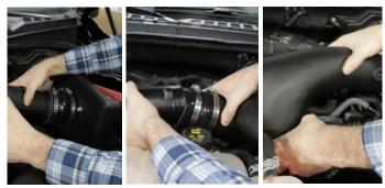
**16.** Install Volant air duct into vehicle by placing the hump hose onto the filter adapter. Then place reducer onto the upper stock inlet. Rotate duct down and into the straight sleeve.
