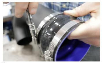
**13.** Install the hump hose onto the Volant air duct along with two #64 clamps and tighten using a ratchet and 8mm socket or flat head screwdriver. Leave clamp on open end of hump hose loose.
