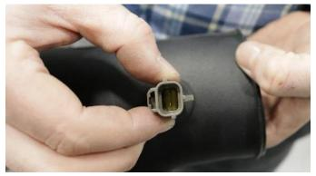
**12.** Install air temp sensor from **Removal Step 9** with the tab facing the short end of the duct, as shown.
