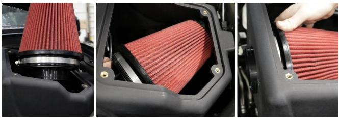
**10.** Insert the filter into the air box with the adapter side down. Rotate the top of the filter down into the air box and rotate the filter around and push the adapter through air box.
