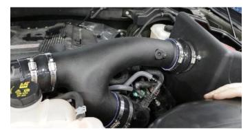
**17.** Adjust air duct as necessary and tighten all clamps using a ratchet and 8mm socket or flat head screw driver. **NOTE:** Make sure to tighten the filter clamp as well.
