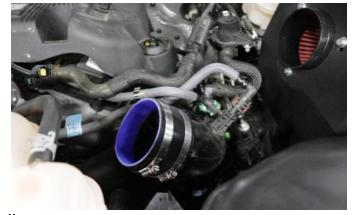
Install the straight sleeve onto lower factory inlet with #64 clamp. Tighten clamp using a ratchet and 8mm socket or flat head screwdriver. Leave clamp on open end of straight sleeve loose.
