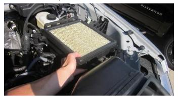
Remove the bottom box assembly by pulling it up and out. Remove the rubber grommet and metal bushing from factory air box. Save for Install Step 1.
