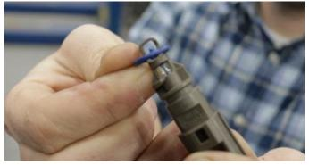
**10.** Remove O-ring from the temp sensor.
