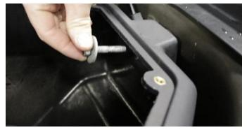
**4.** Attach the Volant air box to the fender with the bolt from Removal Step 4 using a ratchet and 13mm socket.
