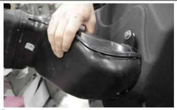
2. Install factory scoop to Volant air box using provided 6mm-25 bolt with flat washers, lock washer, spacer, and nut using 10mm socket or wrench..
